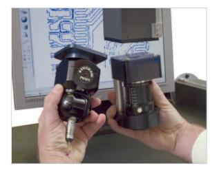
The camera also incorporates a fully programmable 16 LED light ring, which contains alternate white and UV LEDs. The white LEDs provide surface illumination, in the normal manner, whilst the UV LEDs provide an ingenious solution to the perennial problem of backlighting on a CMM: The component to be measured is placed on a plate containing a special reflective paper.
